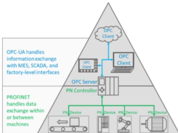
*OPC UA and PROFINET address two different needs in the industrial communication ecosystem. OPC UA used for system monitoring and diagnostics, while PROFINET is used to implement local control loops and processing.*
