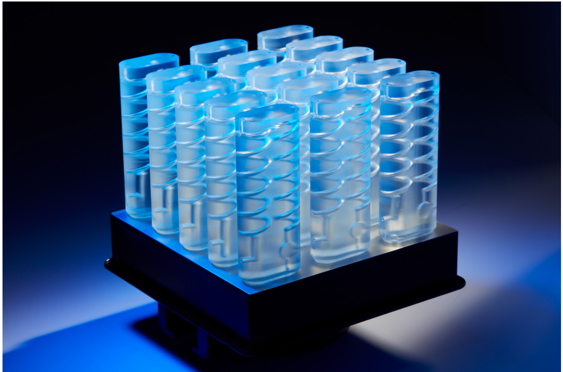
A single large chip prints in just under four hours. A single build platform can print 15 chips of this size at once, in about 24 hours.
